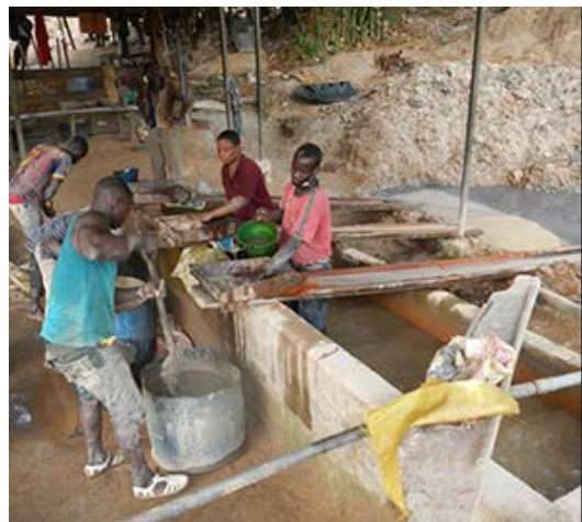
Figure 1. A sluicing station in an artisanal mine. Source: http://www.briloon.org/hgcenter/minamata .
