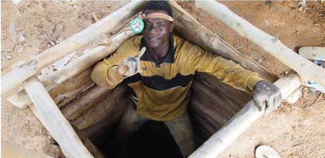
Figure 8. A Ghanaian miner at the opening of a 15-m mine shaft reinforced with wood. Source: https://www.iied.org/ghana-our-way-participatory-reform-artisanal-small-scale-mining-asm-sector .
